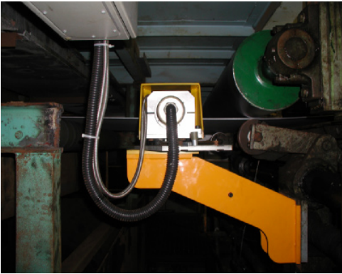
Fig. 9. Installation of CCD camera in plant.
